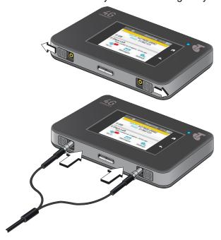
Figure 4. External antennas with TS-9 connectors
