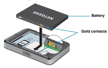
Ensure that the gold contacts on the battery line up with the gold contacts on the device.
