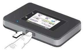
The hotspot powers up and automatically searches for and connects to your network provider's mobile broadband network.
