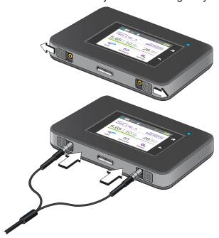
Figure 4. External antennas with TS-9 connectors
