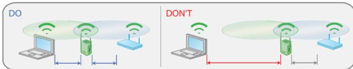
**Tip:** If you have to use a different location, move the Extender closer to the device, but still within the wireless range of the router.
