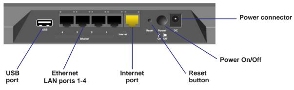
Figure 3. Router, rear view
