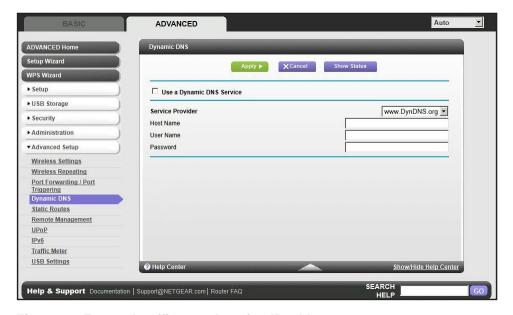
Figure 10. Forward traffic to a changing IP address
