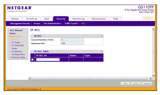
The IP ACL area shows the current size of the ACL table versus the maximum size of the ACL table. The current size is equal to the number of configured IPv4 plus the number of configured MAC ACLs. The maximum size is 100.
