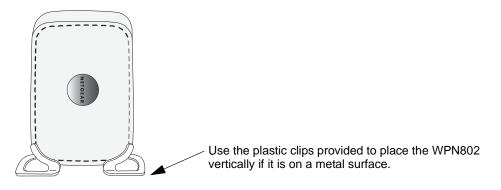
Figure 3-5: WPN802 placed in a vertical orientation
