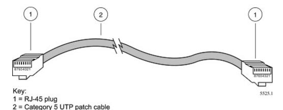
Figure B-3: Category 5 UTP Cable with Male RJ-45 Plug at Each End
