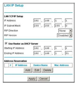
Figure 6-5: LAN IP Setup Menu
