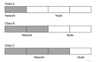
Figure 7-1: Three Main Address Classes
