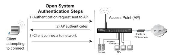
Figure 7-4: Open system authentication
