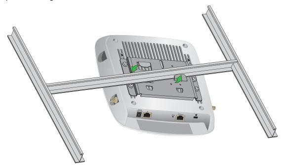
3. Twist the access point to hang it from the ceiling rail.
