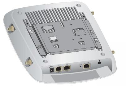
4. So that you can see how the brackets fit together, attach the wall-mounting bracket to the access point–mounting bracket as shown in the following figure.
