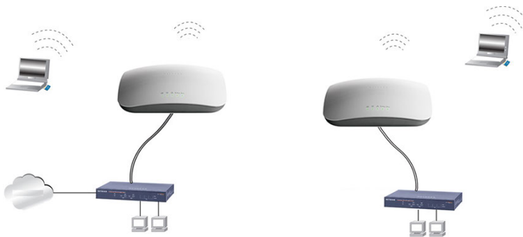
Figure 7. Point-to-point WiFi network
