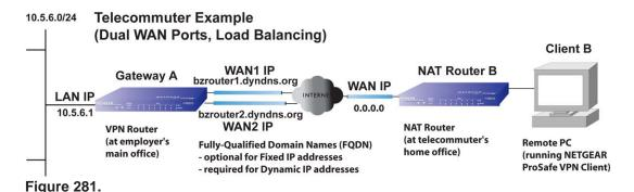
The IP addresses of the gateway WAN ports can be either fixed or dynamic. If an IP address is dynamic, you need to use an FQDN. If an IP address is fixed, an FQDN is optional.
