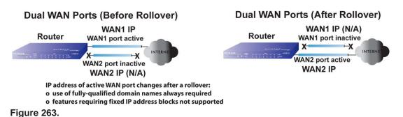
Features such as multiple exposed hosts are not supported in auto-rollover mode because the IP addresses of each WAN port need to be in the identical range of fixed addresses.
