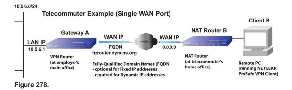
The IP address of the gateway WAN port can be either fixed or dynamic. If the IP address is dynamic, you need to use an FQDN. If the IP address is fixed, an FQDN is optional.
