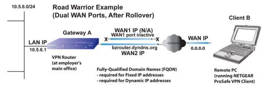
Remote PC must re-establish VPN tunnel after a rollover
