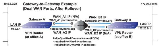
One of the gateway routers must re-establish VPN tunnel after a rollover
