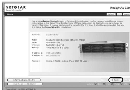
1. In the factory default state, when logged in to the unit, Setup Wizard is enabled. Click **Next** to proceed with the wizard.
