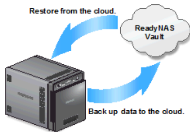
Figure 15. Using a ReadyNAS system to back up and recover data stored on a cloud
