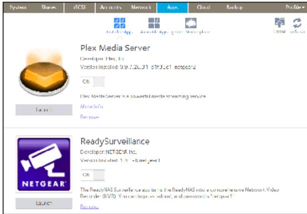
From this window, you can launch, enable, disable, or remove installed apps.
