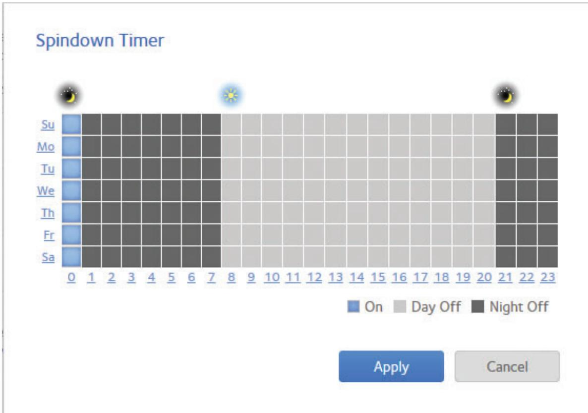
Use the calendar to set the days and times in which spin-down is active. You can set, and the ReadyNAS server will remember, calendar settings whether spin-down is enabled or not.
