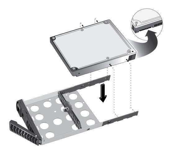
8. Push the mounting bracket and HDD back into the disk tray.
