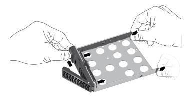
Make sure that the ends of the mounting bracket are even with each other.
