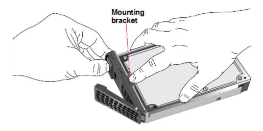
The mounting bracket stops when it hits the bracket lock.
