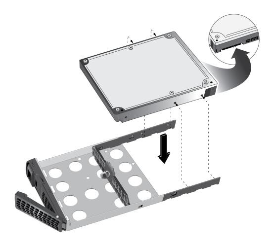
7. Push the mounting bracket and HDD back into the disk tray.
