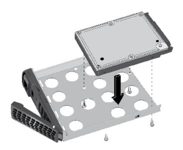
Make sure that the HDD or SSD is installed on the correct side of the disk tray.
