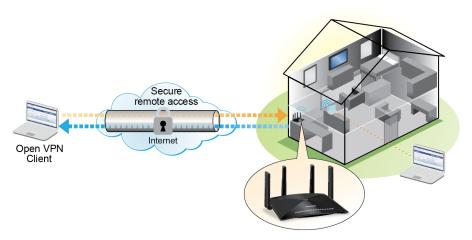
This type of VPN access is called a client-to-gateway tunnel. The computer is the client, and the router is the gateway. To use the VPN feature, you must log in to the router and enable VPN, and you must install and run VPN client software on the computer.
