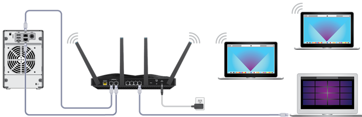
Figure 11. Ethernet port aggregation
