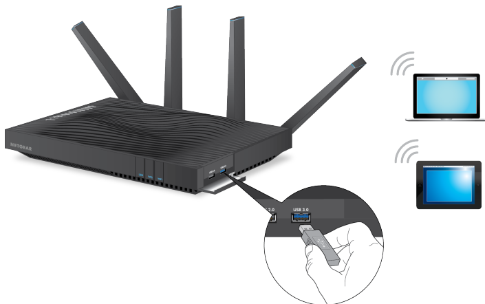
Figure 14. A USB 3.0 and USB 2.0 port are located on the side of the router
