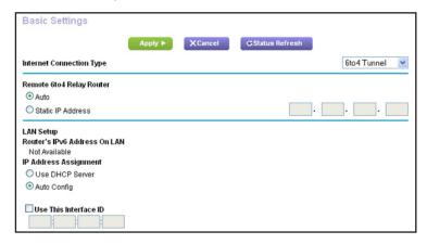
The router automatically detects the information in the Router's IPv6 Address on LAN field. This field shows the IPv6 address that is acquired for the router's LAN interface. The number after the slash (/) is the length of the prefix, which is also indicated by the underline (\_) under the IPv6 address. If no address is acquired, the field displays Not Available.
