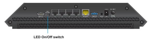
The Power LED stays lit even if the **LED On/Off** switch is in the Off position.
