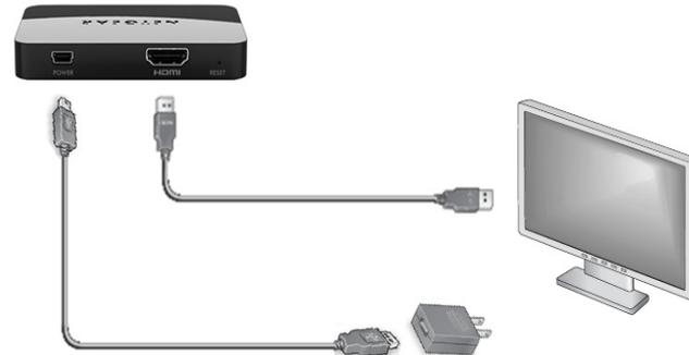
The Push2TV adapter LED is blinking when the adapter powers up. The LED turns solid to indicate that the adapter is ready, but is not yet connected to your computer.
