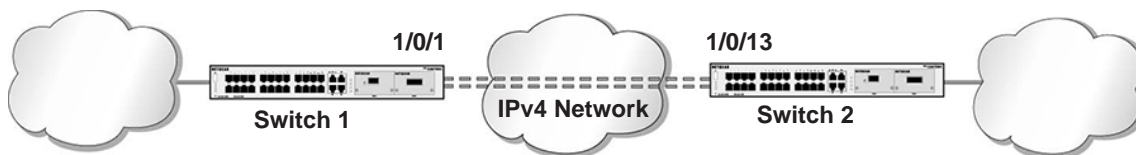
Figure 56. 6in4 tunnel configuration
