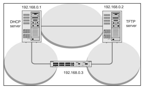
Figure 1. Components in an Auto Install configuration
