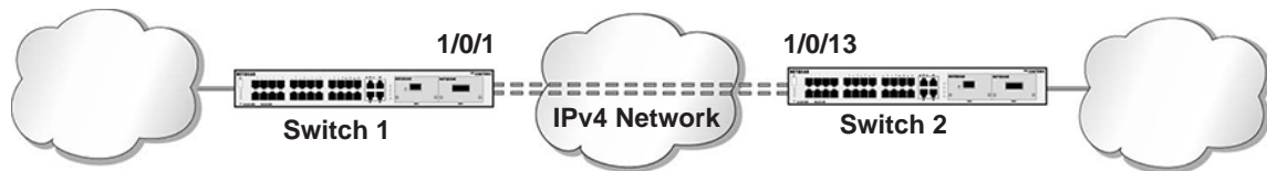
Figure 55. 6in4 tunnel configuration
