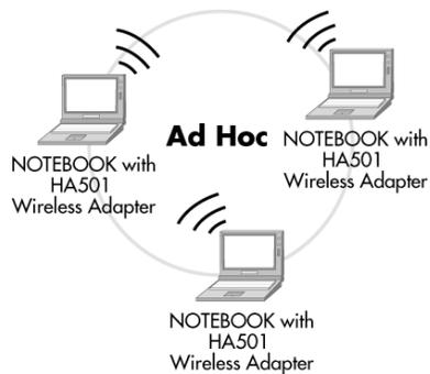
In this configuration, network packets are directly sent and received by the intended transmitting and receiving stations. As long as the stations are within range of one another, this is the easiest and least expensive way to set up a wireless network.
