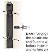
**Note:** For drywall, use the plastic anchors and fold the wings in before inserting an anchor into a wall.
