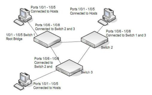
Figure 4. MSTP example configuration
