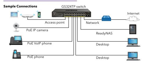
This section applies only to switch model GS324TP. This switch can supply up to 30W PoE+ (IEEE 802.3at) to each copper port, with a total maximum PoE power budget of 190W across all active PoE+ ports.
