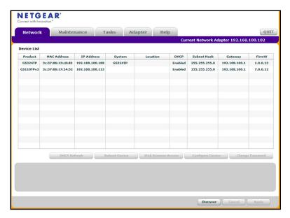
**6.** Write down the switch IP address assigned by the DHCP server.
