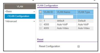
7. In the VLAN ID field, specify the VLAN identifier for the new VLAN.
