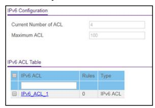
7. In the IPv6 ACL field, specify a name to identify the IPv6 ACL.
