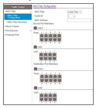
The previous figure shows the MAC Filter Configuration page for model GS110TPv3.
