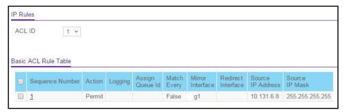
If no rules exist, the Basic ACL Rule Table might show the message *No rules were* configured for this ACL. If one or more rules exist for the ACL, the rules display in the Basic ACL Rule Table.
