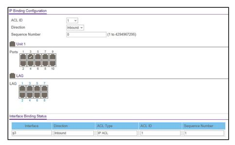
The previous figure shows the IP Binding Configuration page for model GS110TPv3.
