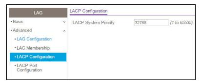
7. In the LACP System Priority field, specify the switch's link aggregation priority relative to the devices at the other ends of the links on which link aggregation is enabled.
