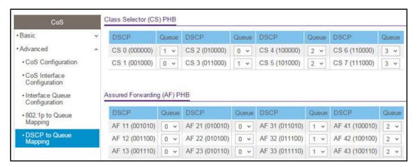
**7.** For each DSCP value, select from the corresponding **Queue** menu which internal traffic class must be mapped to the DSCP value.
