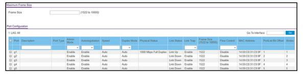
7. In the **Frame Size** field, specify the maximum Ethernet frame size that each interface can support.
