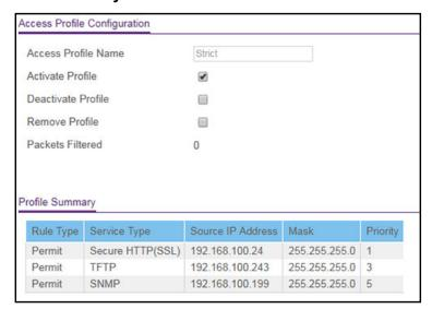
The Packets Filtered field displays the number of packets filtered (none in the previous figure).
