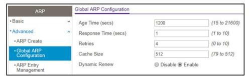
**7.** In the **Age Time** field, enter the time, in seconds, that a dynamic ARP entry remains in the ARP table before aging out.
