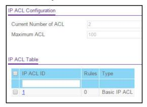
The IP ACL page shows the current size of the ACL table compared to the maximum size of the ACL table. The current size is equal to the number of configured IPv4 ACLs plus the number of configured MAC ACLs and IPv6 ACLs. The maximum number of ACLs on the switch is 100.
