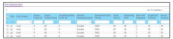
The previous figure shows only part of the page for models GS108Tv3 and GS110TPv3. Model GS110TPP also supports MAC-based Authentication Bypass (MAB) and includes a MAB column to the right of the Port Control column.
