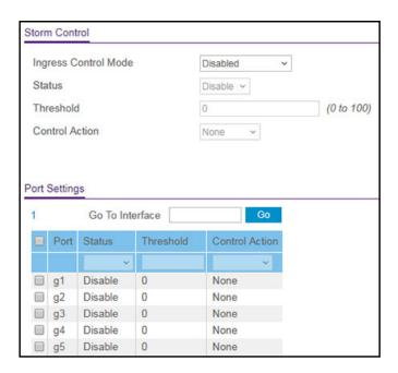
The default settings in the Port Settings section depends on the global storm control settings (see Configure global storm control settings on page 344), which apply to all ports.
