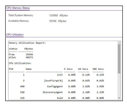
The CPU Utilization section shows the memory information, task-related information, and percentage of CPU utilization per task.
