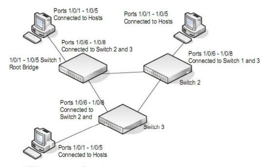
Figure 4. MSTP example configuration
