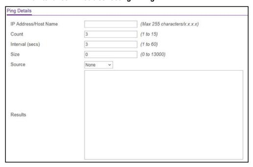
7. In the IP Address/Host Name field, enter the IP address or host name of the device that must be pinged.
