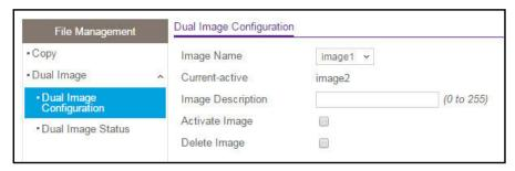
**7.** From the **Image Name** menu, select the image that is *not* the image displayed in the Current-active field but that is the image that you want the switch to run *after* it reboots.
