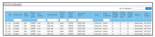
The previous figure shows the PoE Port Configuration page for model GS110TPv3.
