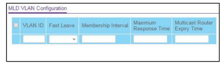
7. In the VLAN ID field, specify the VLAN IDs for which MLD snooping is enabled.
