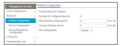
The Current Server IP Address field is blank if no servers are configured (see <u>Configure a RADIUS authentication server on the switch on page 298</u>). The switch supports up to three RADIUS servers. If more than one RADIUS server is configured, the current server is the server configured as the primary server. If no servers are configured as the primary server, the current server is the most recently added RADIUS server.
