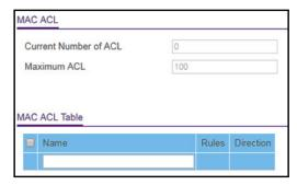
The MAC ACL Table displays the number of ACLs currently configured in the switch and the maximum number of ACLs that can be configured. The current size is equal to the number of configured IPv4 and IPv6 ACLs plus the number of configured MAC ACLs.
