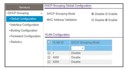
7. Select the DHCP Snooping Mode **Enable** radio button.
