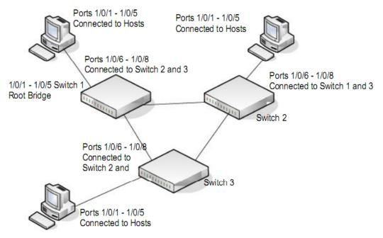
Figure 2. MSTP sample configuration
