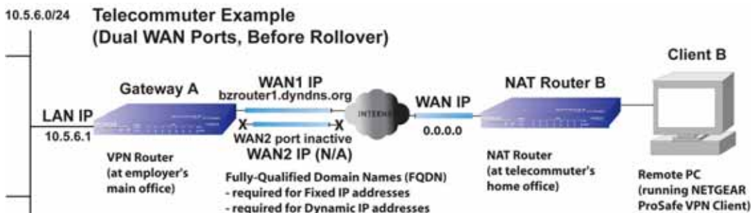
Figure 29. Telecommuter example in a dual WAN port configuration with NAT before auto-rollover
