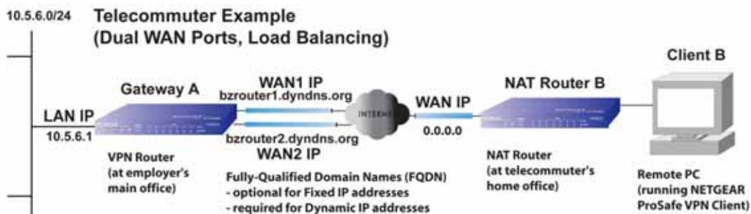
Figure 31. Telecommuter example in a dual WAN port configuration with NAT and load balancing
