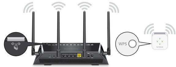
1. Press the **WPS** button on the extender until the WPS LED blinks.
