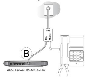
Figure 3-5: Connecting the DG834 ADSL router to an ADSL microfilter and phone
