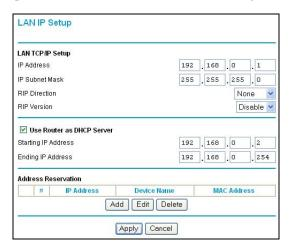
Figure 6-2: LAN IP Setup Menu
