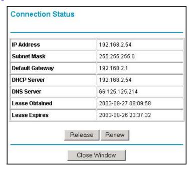
Figure 5-5: Connection Status screen for Dynamic IP
