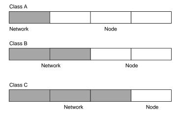
Figure 7-1: Three Main Address Classes
