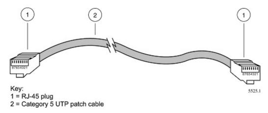
Figure B-3: Category 5 UTP Cable with Male RJ-45 Plug at Each End
