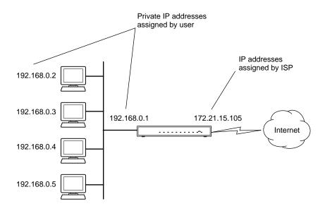
Figure 7-3: Single IP Address Operation Using NAT
