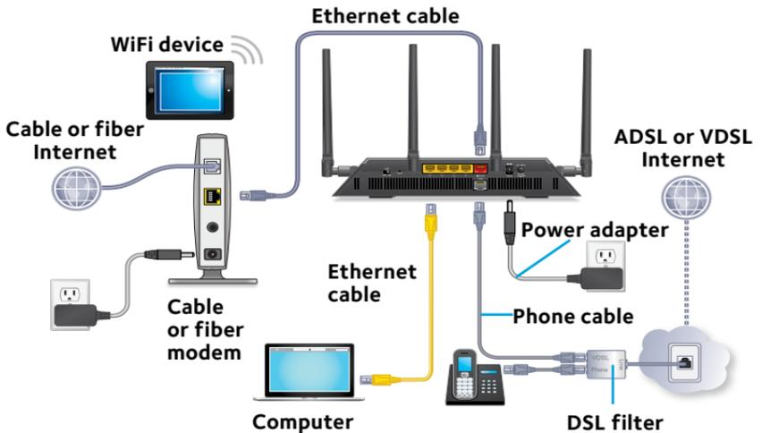
You can use a wired connection to connect a computer to the modem router, or you can use a WiFi connection to connect a computer or WiFi device to the modem router:
