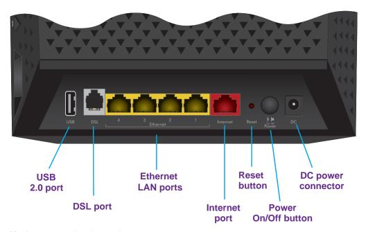
Figure 3. Modem router back panel
