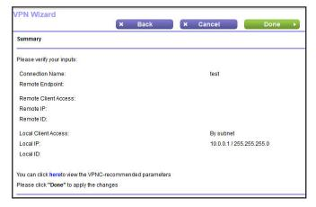
This screen shows the summary of the Wizard configuration with a link to view the VPNC recommended parameters (click the **here** link to view the VPNC-recommended parameters).
