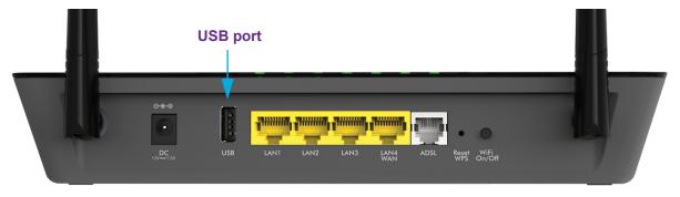
Figure 10. USB port on the back panel
