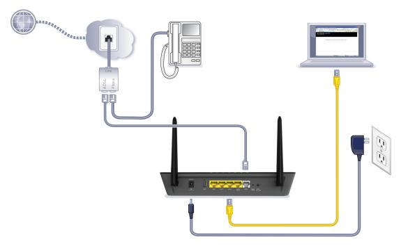
Figure 7. Modem router cabling for DSL service
