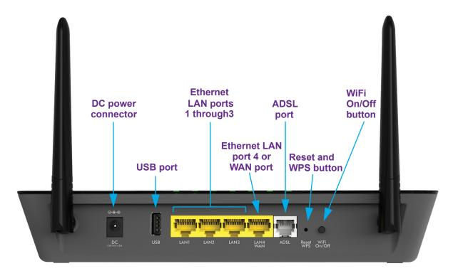
Figure 3. Modem router back panel
