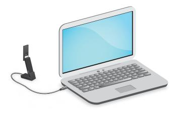
**Note:** When the adapter is placed in the desktop dock, you can fold out the adapter to its maximum angle for increased WiFi performance.
