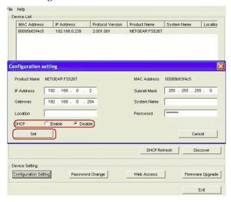
Figure 3-4: Assigning the switch a static IP address
