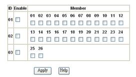
Port Trunking is a feature that allows multiple links between switches to work as one virtual link (aggregate link). Trunks can be defined for similar port types only. For example, a 10/100 port cannot form a Port Trunk with a gigabit port. For 10/100 ports, trunks can only be formed within the same bank. A bank is a set of eight ports, such as ports 1 to 8, ports 9 to 16, ports 17 to 24, or port 25 and port 26, on the same switch unit. Up to four trunks can be operating at the same time.
