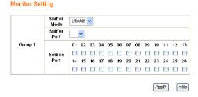
The Monitor feature allows you to configure any port's incoming and/or outgoing traffic to be mirrored to a pre-defined sniffer port.
