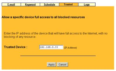
To specify a Trusted Host, enter the Trusted Host's IP address in the Trusted Device box and click Apply.
