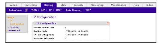
**b.** For Routing Mode, select the **Enable** radio button.
