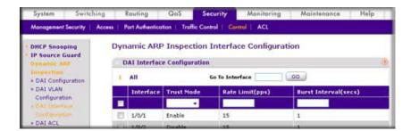
Now ARP packets from the DHCP client will go through; however ARP packets from the static client are dropped, since it does have a DHCP snooping entry. It can be overcome by static configuration as described in the following section, *Static Mapping* on page 357.
