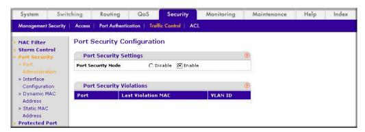
**b.** Under Port Security Configuration, next to Port Security Mode, select the **Enable** radio button.
