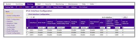
**b.** Under IPv6 Interface Configuration, scroll down and select the Interface **2/0/21** check box.
