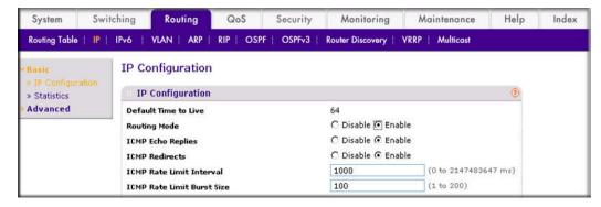
**b.** For Routing Mode, select the **Enable** radio button.
